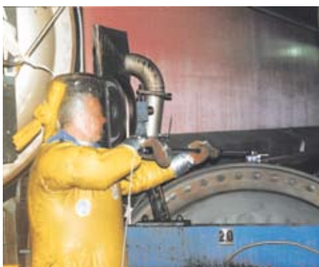
SWT 315, surface temperature of a drying cylinder.
