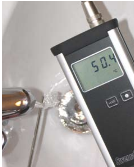
Tap water temperature with SwemaTemp 20 with T51
